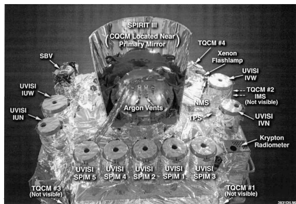
Fig. 3 Photograph of instrument section of MSX (+X direction).
